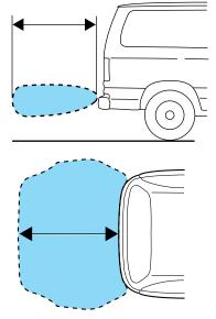
The RSS automatically turns on when the gearshift lever is placed in R (Reverse) and the ignition is on. An RSS control allows the driver to turn the RSS on and off. To turn the RSS off, the ignition must be ON, and the gear selector in R (Reverse). An indicator light on the
