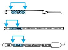
The transmission fluid should be in this range if at ambient temperature (50°F-95°F [10°C-35°C]).
