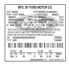
**WARNING:** Exceeding the Safety Compliance Certification Label vehicle weight rating limits could result in substandard vehicle handling or performance, engine, transmission and/or structural damage, serious damage to the vehicle, loss of control and personal injury.
