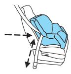
10. Try to pull the belt out of the retractor to make sure the retractor is in the automatic locking mode (you should not be able to pull more belt out). If the retractor is not locked, unbuckle the belt and repeat Steps 2 through 9.
