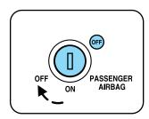
**WARNING:** If the light fails to illuminate when the passenger air bag switch is in the OFF position and the ignition switch is in ON, have the passenger air bag switch serviced at your Ford or Lincoln-Mercury dealer immediately.
