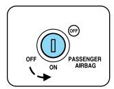
**WARNING:** If the OFF light is illuminated when the passenger airbag switch is in the ON position and the ignition switch is in ON, have the passenger airbag switch serviced at an authorized dealer immediately.
