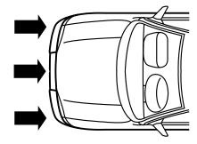
near-frontal collisions, not rollover, side-impact, or rear-impacts unless the collision causes sufficient longitudinal deceleration.
