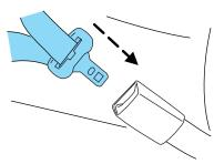
Grasp the shoulder portion and pull downward until the entire belt is pulled out.
