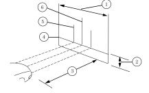
or cross marker) or on the bulb shield, internal to the lamp (mark or feature). Measure the height from the center of your headlamp to the ground (2) and mark an 8 foot (2.4 meter) long horizontal line on the wall or screen (1) at this height (masking tape works well).
