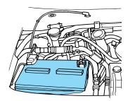
**WARNING:** This vehicle may be equipped with more than one battery, removal of cable from only one battery does not disconnect the vehicle electrical system. Be sure to disconnect cables from all batteries when disconnecting power. Failure to do so may cause serious personal injury or property damage.
