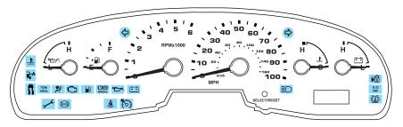
Warning lights and gauges can alert you to a vehicle condition that may become serious enough to cause expensive repairs. A warning light may illuminate when a problem exists with one of your vehicle's functions. Many lights will illuminate when you start your vehicle to make sure the bulb works. If any light remains on after starting the vehicle, refer to the respective system warning light for additional information.
