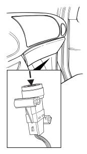
On commercial stripped chassis vehicles, this switch is located on a bracket above the brake pedal.
