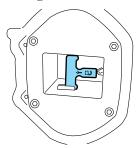
• The rear door handle is located in the rear door below the glass.
