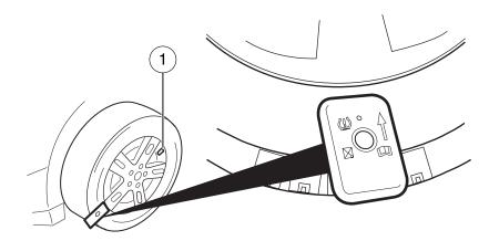
1. **Left front tire:** Place the TPMS reset tool against the left front tire where the tire meets the rim, opposite from the valve stem (1) as shown. This is where the sensor is located inside the rim.
