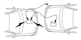
$2.\ \mbox{Remove}$  the jumper cable on the negative (-) connection of the booster vehicle's battery.
