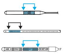
The transmission fluid should be in this range if at normal operating temperature (150°F-170°F [66°C-77°C]).
