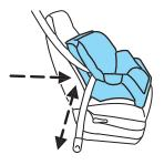
be no more than one inch (2.5 cm) of movement for proper installation.
