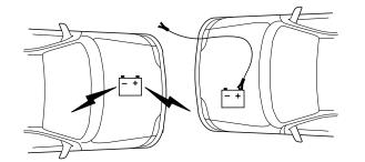
1. Connect the positive (+) jumper cable to the positive (+) terminal of the discharged battery.
