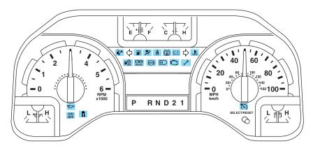
Warning lights and gauges can alert you to a vehicle condition that may become serious enough to cause expensive repairs. A warning light may illuminate when a problem exists with one of your vehicle's functions. Many lights will illuminate when you start your vehicle to make sure the bulb works. If any light remains on after starting the vehicle, refer to the respective system warning light for additional information.
