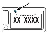
To use the camera system, place the transmission in R (Reverse); an image will display on the left portion of the rear view mirror or on the navigation screen (if equipped). The area displayed on the screen may vary according to the vehicle orientation and/or road condition.
