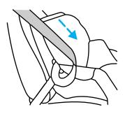
9. Attach the tether strap (if the child seat is equipped). Refer to *Attaching child safety seats with tether straps* later in this chapter.
