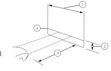
5. Locate the vertical adjuster on the back of each headlamp, then use a long Phillips #2 screwdriver to turn the adjuster either counterclockwise (to adjust down) or clockwise (to adjust up) aligning the upper edge of the light pattern up to the horizontal line.
