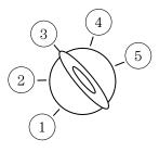
3. Within 10 seconds of removing the first **coded key**, insert the second previously programmed **coded key** into the ignition and turn the ignition from the 3 (off) position to the 4 (on) position (maintain ignition in the 4 (on) position for at least one second but no more than 10 seconds).
