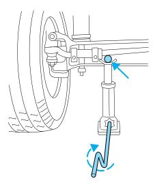
5. Remove the jack and fully tighten the lug nuts in the following pattern (Refer to *Wheel lug nut torque specifications* later in this chapter for the proper lug nut torque specification):
