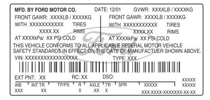
**GVWR (Gross Vehicle Weight Rating)** – is the maximum allowable weight of the fully loaded vehicle (including all options, equipment, passengers and cargo). **The GVWR is shown on the Safety Compliance Certification Label located on the B-Pillar or the edge of the driver's door. The GVW must never exceed the GVWR.**
