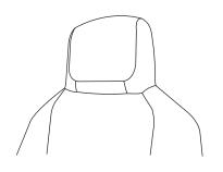
Properly adjust the seatback to an upright driving/riding position, so that the head restraint is positioned as close as possible to the back of your head.
