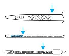
Fluid levels above the safe range may result in transmission failure. An overfill condition of transmission fluid may cause shift and/or engagement concerns and/or possible damage.
