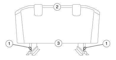
4. With assistance, pull the LH/RH seat latch release straps (1) (located behind the latch mechanisms) to release the latch from the rear strikers.
