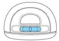
With the ignition key in the accessory or on position, the rear lamp can be turned on or off by sliding the control.
