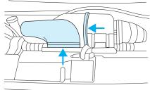
3. Carefully separate the two halves of the air filter housing.
