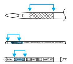
The transmission fluid should be in this range if at ambient temperature (50°F-95°F [10°C-35°C]).
