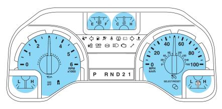
**Speedometer:** Indicates the current vehicle speed.
