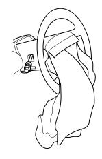
serious injuries such as fractures, facial and eye injuries or internal injuries, particularly to occupants who are not properly restrained or are otherwise out of position at the time of airbag deployment. It is extremely important that occupants be properly restrained as far away from the airbag module as possible while maintaining vehicle control.
