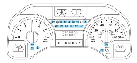
Warning lights and gauges can alert you to a vehicle condition that may become serious enough to cause expensive repairs. A warning light may illuminate when a problem exists with one of your vehicle's functions. Many lights will illuminate when you start your vehicle to make sure the bulb works. If any light remains on after starting the vehicle, refer to the respective system warning light for additional information.
