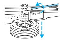
To stow the cable retainer with the spare removed, turn the jack handle clockwise until all slack is removed.
