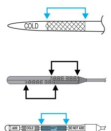
If an overfill occurs, excess fluid should be removed by an authorized dealer
