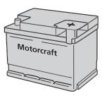
**WARNING:** This vehicle may be equipped with more than one battery, removal of cable from only one battery does not disconnect the vehicle electrical system. Be sure to disconnect cables from all batteries when disconnecting power. Failure to do so may cause serious personal injury or property damage.
