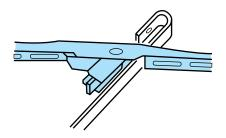
Replace wiper blades at least once per year for optimum performance. Poor wiper quality can be improved by cleaning the wiper blades and the windshield. Refer to *Windows and wiper blades* in the *Cleaning* chapter. To prolong the life of the wiper blades, it is highly recommended to scrape off the ice on the windshield before turning on the wipers. The layer of ice has many sharp edges and can damage the micro edge of the wiper rubber element.
