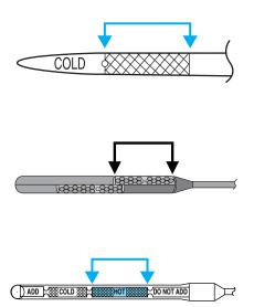
The transmission fluid should be in this range if at normal operating temperature (150°F-170°F [66°C-77°C]).
