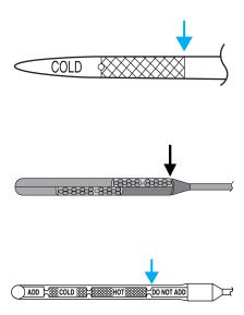
Fluid levels above the safe range may result in transmission failure.
