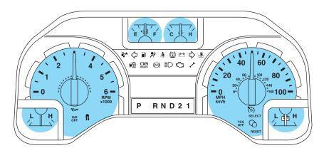
**Speedometer:** Indicates the current vehicle speed.
