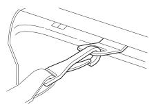
3. Tighten the child safety seat tether strap according to the manufacturer's instructions.
