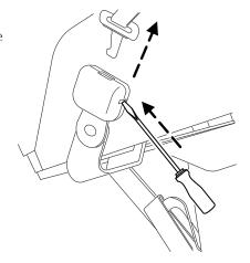
2. Find the clips attached near the ends of the lap/shoulder belts.
