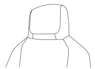
Properly adjust the seatback to an upright driving/riding position, so that the head restraint is positioned as close as possible to the back of your head
