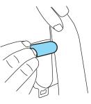
The end of the shoulder belt **must** be clipped in order to keep it from striking anything during vehicle operation.
