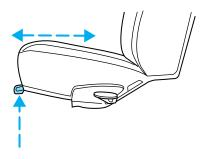
5. Tighten the child safety seat tether strap according to the manufacturer's instructions.
