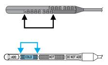
The transmission fluid should be in this range if at ambient temperature (50°F-95°F [10°C-35°C]).
