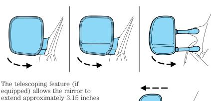
equipped) allows the mirror to extend approximately 3.15 inches (80 mm). This feature is especially useful to the driver when towing a trailer.
