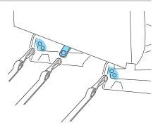
If the tether strap is clipped incorrectly, the child safety seat may not be retained properly in the event of a collision.
