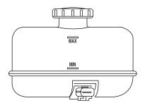
The fluid level will drop slowly as the brakes wear, and will rise when the brake components are replaced. Fluid levels between the MIN and MAX lines are within the normal operating range; there is no need to add fluid. If the fluid levels are outside of the normal operating range, the performance of the system could be compromised; seek service from your authorized dealer immediately.
