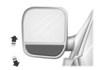
You can tilt the spotter mirror up or down to increase visibility. Only apply pressure to the center of the top or bottom edges when adjusting the mirror.
