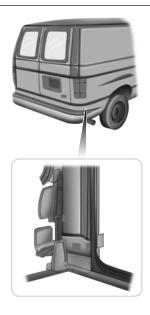
• The jack is located in the rear right-hand side of the cargo area.
