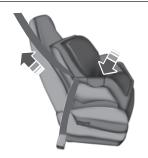
8. Remove remaining slack from the belt. Force the seat down with extra weight, for example, by pressing down or kneeling on the child restraint while pulling up on the shoulder belt in order to force slack from the belt.
