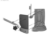
1. Turn the headlamp switch to the off position, then remove the four screws and the lamp assembly from the vehicle.
