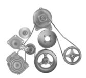
$\bullet\,$  4.6L V8, 5.4L V8 and 6.8L V10 engines with A/C
