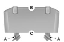
4. With assistance, pull the seat latch release straps (A) (located behind the latch mechanisms) to release the latch from the rear strikers.
