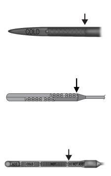
Fluid levels above the safe range may result in transmission failure. An overfill condition of transmission fluid may cause shift and/or engagement concerns and/or possible damage.
