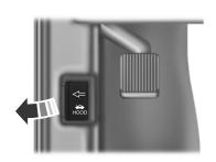
1. Inside the vehicle, pull the hood release handle located under the bottom left corner of the instrument panel.
