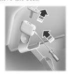
1. Disengage the lap and shoulder belt from the seat by inserting a key or small screwdriver into the slot in the detachable anchor and lifting upward.
