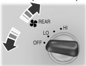
Controls the volume of air circulated in the rear of your vehicle. Adjust to select the desired fan speed or switch off.
