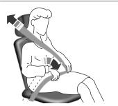
Pregnant women should always wear their safety belts. The lap belt portion of a combination lap and shoulder belt should be positioned low across the hips below the belly and worn as tight as comfort will allow. The shoulder belt should be positioned to cross the middle of the shoulder and the center of the chest.
