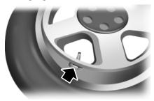
**Note:** Each road tire is equipped with a tire pressure sensor located inside the tire and wheel assembly cavity. The pressure sensor is attached to the valve stem. The pressure sensor is covered by the tire and is not visible unless the tire is removed. Take care when changing the tire to avoid damaging the sensor.
