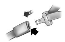
2. To unfasten, press the release button and remove the tongue from the buckle.
