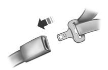
1. Insert the belt tongue into the proper buckle (the buckle closest to the direction the tongue is coming from) until you hear a snap and feel it latch. Make sure the tongue is securely fastened in the buckle.
