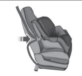
3. While holding the shoulder and lap belt portions together, route the tongue through the child seat according to the child seat manufacturer's instructions. Be sure the belt webbing is not twisted.
