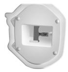
• The side door emergency handle is located on the door inner trim panel in the speaker cup.
