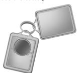
1. Twist a thin coin between the two halves of the remote entry transmitter near the key ring.
