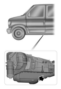
The TorqShift® automatic transmission is equipped with a serviceable transmission fluid filter located inside the transmission bottom pan.
