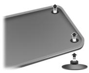
**WARNING:** Always use floor mats that are designed to fit the footwell of your vehicle. Only use floor mats that leave the pedal area unobstructed. Only use floor mats that are firmly secured to retention posts so that they cannot slip out of position and interfere with the pedals or impair safe operation of your vehicle in other ways.
