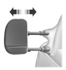
This feature allows the mirror to extend approximately 3 inches (80 millimeters). It is especially useful when towing a trailer.
