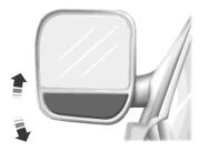
You can tilt the spotter mirror up or down to increase visibility. Only apply pressure to the center of the top or bottom edges when adjusting the mirror.
