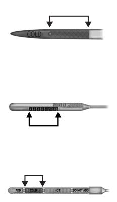
The transmission fluid should be in this range if at ambient temperature (50°F-95°F [10°C-35°C]).
