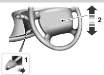
1. Pull and hold the steering wheel release lever.
