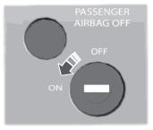
1. Insert the ignition key and turn the switch to on.
