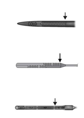
Fluid levels above the safe range may result in transmission failure. An overfill condition of transmission fluid may cause shift and/or engagement concerns and/or possible damage.
