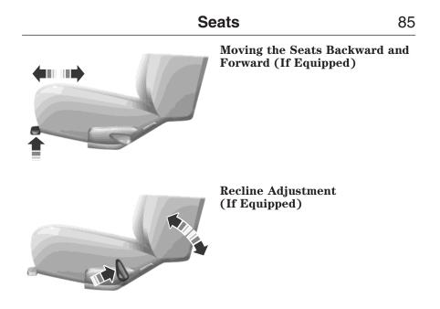
**WARNING:** Before returning the seatback to its original position, make sure that cargo or any objects are not trapped behind the seatback. After returning the seat back to its original position, pull on the seatback to make sure that it has fully latched. An unlatched seat may become dangerous in the event of a sudden stop or crash.
