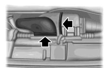
1. Disconnect the fresh air inlet tube from the radiator support.
