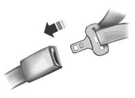
1. Insert the belt tongue into the proper buckle (the buckle closest to the direction the tongue is coming from) until you hear a snap and feel it latch. Make sure the tongue is securely fastened in the buckle.
