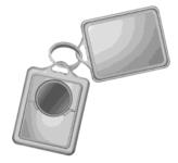
1. Twist a thin coin between the two halves of the remote entry transmitter near the key ring. **Note:** Do not take the rubber cover and circuit board off the front housing of the remote entry transmitter.
