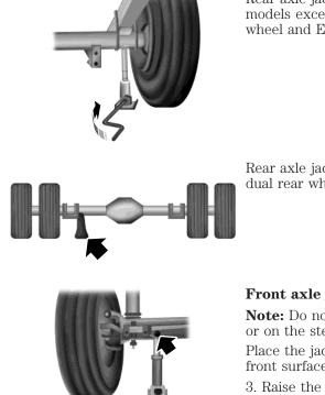
Rear axle jacking points - All models except E-350 dual rear wheel and E-450
