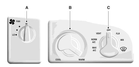
A. **Fan speed control:** Controls the volume of air circulated in your vehicle. Adjust to select the desired fan speed.
