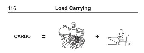
**Cargo Weight** – includes all weight added to the Base Curb Weight, including cargo and optional equipment. When towing, trailer tongue load or king pin weight is also part of cargo weight.
