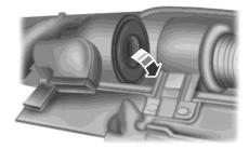
3. Carefully separate the two halves of the air filter housing.4. Remove the air filter element from the housing.
