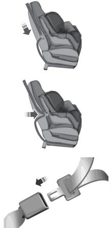
2. Pull down on the shoulder belt and then grasp the shoulder belt and lap belt together.
