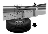
5. Remove the jack handle from the right side compartment and insert the tip of the jack handle through the access hole and into the tube.
