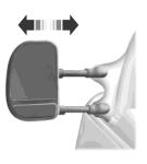
This feature allows the mirror to extend approximately 3 inches (80 millimeters). It is especially useful when towing a trailer.
