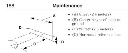
2. Measure the height from the center of your headlamp (indicated by a 3.0 millimeter circle on the lens) to the ground and mark an 8 foot (2.4 meter) horizontal reference line on the vertical wall or screen at this height (a piece of masking tape works well).
