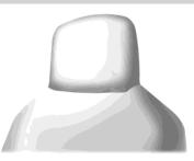
The front row outboard non-adjustable head restraints consist of a trimmed foam covering over the upper structure of the seatback. Properly adjust the seatback to an upright driving or riding position, so that the head restraint is positioned as close as possible to the back of your head.
