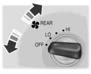
Controls the volume of air circulated in the rear of your vehicle. Adjust to select the desired fan speed or switch off.
