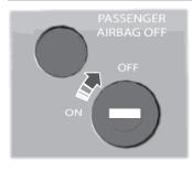
1. Insert the ignition key, turn the switch to off, and hold it in the off position while removing the key.
