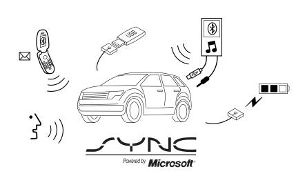
SYNC is an in-vehicle communications system that works with your Bluetooth-enabled cellular phone and portable media player. This allows you to:
