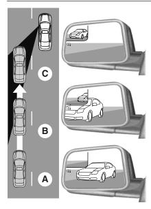
The image of the approaching vehicle is small and near the inboard edge of the main mirror when it is at a distance. The image becomes larger and begins to move outboard across the main mirror as the vehicle approaches (A). The image will transition from the main mirror and begin to appear in the blind spot mirror as the vehicle approaches (B). The vehicle will transition to your peripheral field of view as it leaves the blind spot mirror (C).
