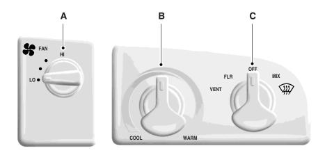
A. **Fan speed control:** Controls the volume of air circulated in your vehicle. Adjust to select the desired fan speed.
