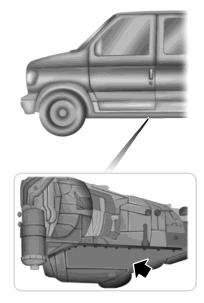
The TorqShift® automatic transmission is equipped with a serviceable transmission fluid filter located inside the transmission bottom pan.
