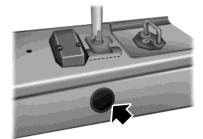
3. To remove the spare tire, remove the thumb screw and anti-theft bracket. If finger pressure will not remove the thumb screw, use the lug wrench to loosen the screw.
