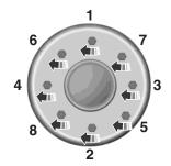
8. Remove the jack and fully tighten the lug nuts in the following pattern. See *Wheel Lug Nut Torque Specifications*.
