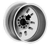
**Note:** Inspect the wheel pilot hole and mounting surface prior to installation. Remove any visible corrosion or loose particles.
