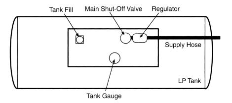
The regulator reduces the pressure of the propane gas vapor from the pressure in the tank, to the pressure required for use at the appliances. This reduction in pressure is performed by a two-stage regulator. Two regulators are used in the same body to reduce the pressure of the propane gas in the tank for use by the appliances in the motorhome. The regulator seldom requires service, but it should always be protected from the elements and extremes of hot and cold.
