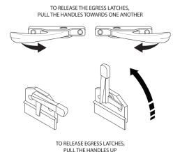
An egress window is designated for use as an exit in the case of an emergency. Inside the motorhome the egress window is easily identified by the red locking handles. There are two common styles of latches, determine the style of locking handle you have and refer to the following illustrations for operation. It is also marked as an "EXIT". The glass slider in the egress window operates the same as all other windows;
