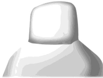
The front row outboard non-adjustable head restraints consist of a trimmed foam covering over the upper structure of the seatback. Properly adjust the seatback to an upright driving or riding position, so that the head restraint is positioned as close as possible to the back of your head.
