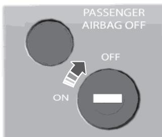
1. Insert the ignition key, turn the switch to off, and hold it in the off position while removing the key.
