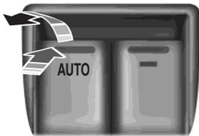
Press the switch to open the window.
