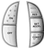
The cruise controls are located on the steering wheel.
