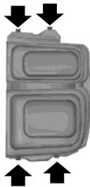
2. Remove the four screws from the headlamp assembly and carefully remove the lamp/bezel.
