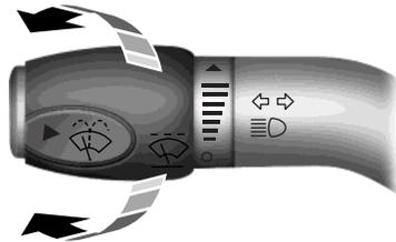
Rotate the end of the control:
