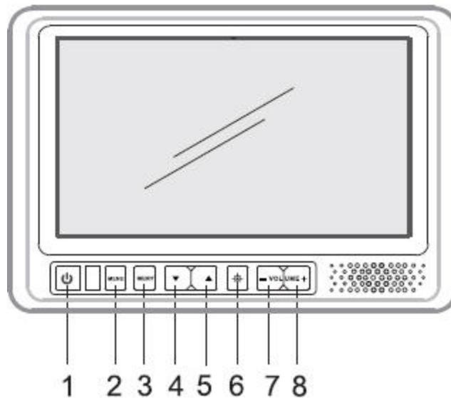
1. Power On/Off: Press once turns unit on.
