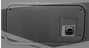
The furnaces used by Thor Motor Coach have electronic ignition, and there is no need to access this panel except for service. As with all appliances, service is best left for your dealer. To remove the panel to check for insect nests, you will need a Square or a Phillips head screwdriver. For further information, reference the furnace manufacturer's manual provided with your vehicle.
