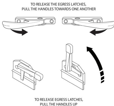
An egress window is designated for use as an exit in the case of an emergency. Inside the motorhome the egress window is easily identified by the red locking handles. There are two common styles of latches, determine the style of locking handle you have and refer to the following illustrations for operation. It is also marked as an "EXIT". The glass slider in the egress window operates the same as all other windows;
