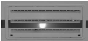
The refrigerator is an electronic ignition appliance and there is no need to access this panel except for service or checking for insect nests. If a problem is encountered, follow the guidelines for use as outlined in the Refrigerator Owner's Manual located in the Owner's Information Kit. If the problem is not resolved, contact an authorized Thor Motor Coach dealer.
