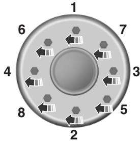
8. Remove the jack and fully tighten the lug nuts in the following pattern. See *Wheel Lug Nut Torque Specifications* in this chapter for the proper lug nut torque specification.
