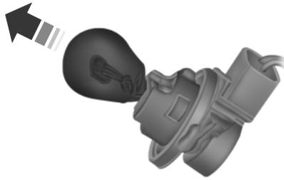
2. Rotate the bulb socket counterclockwise and remove it from lamp assembly.
