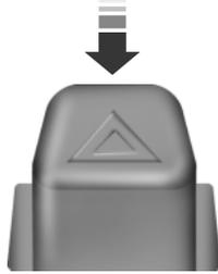
The hazard flasher is located on the steering column, just behind the steering wheel. The hazard flashers will operate when the ignition is in any position or if the key is not in the ignition.
