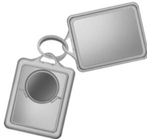
1. Twist a thin coin between the two halves of the remote entry transmitter near the key ring.
