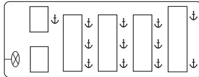
For the center position of a three-passenger bench seat, attach the tether strap directly to the tether bracket provided under the back edge of the seat cushion. For the outboard positions, attach the tether strap to the slot in the side of the seat pedestal.
