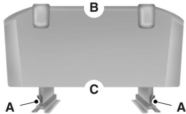
4. With assistance, pull the seat latch release straps (A) (located behind the latch mechanisms) to release the latch from the rear strikers.
