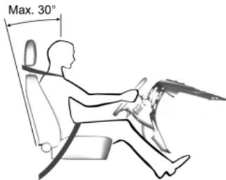
When you use them properly, the seat, head restraint, safety belt and airbags will provide optimum protection in the event of a crash. We recommend that you follow these guidelines:
