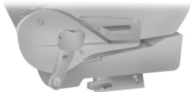
2. Pull the seat latch handle, then pull the seat toward the right side of the vehicle to disengage four pins from the floor mount.
