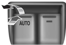
Press the switch to open the window.
