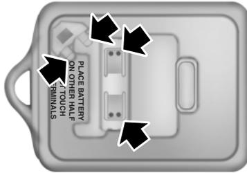
2. Do not wipe off any grease on the battery terminals on the back surface of the circuit board.
