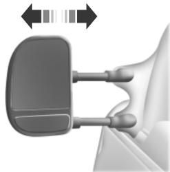
This feature allows the mirror to extend approximately 3 inches (80 millimeters). It is especially useful when towing a trailer.
