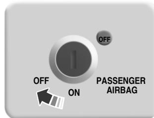
1. Insert the ignition key, turn the switch to off, and hold it in the off position while removing the key.
