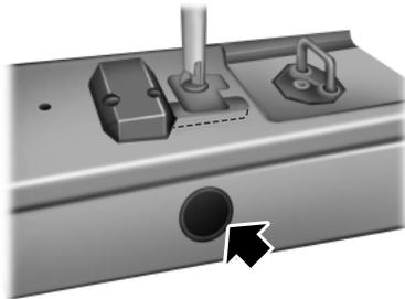
1. Open the rear doors and remove the thumb screw and anti-theft bracket. If finger pressure will not remove the thumb screw, use the lug wrench to loosen the screw.
