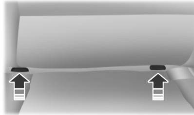
The LATCH lower anchors are located at the rear section of the rear seat between the cushion and seatback.
