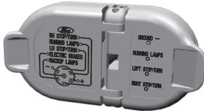
When attaching the trailer wiring connector to your vehicle, only use a proper fitting connector that works with the vehicle and trailer functions. If your vehicle has a trailer towing package, it may have a 7-pin connector. Some connectors may have the SAE J2863 logo, which confirms that it is the proper wiring connector and works correctly with your vehicle.
