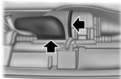
1. Disconnect the fresh air inlet tube from the radiator support.
