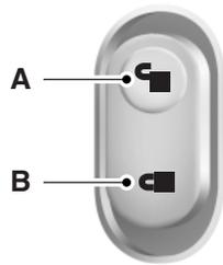
The passenger side rear cargo door has a lock control mounted on the inside of the door. Press to unlock or lock all the doors.
