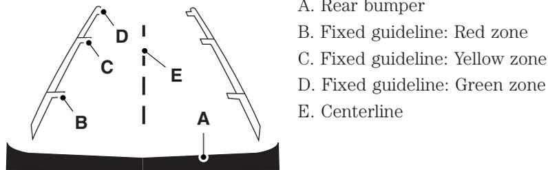
The fixed guidelines fade in and out depending on the steering wheel position.
