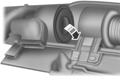
3. Carefully separate the two halves of the air filter housing.
