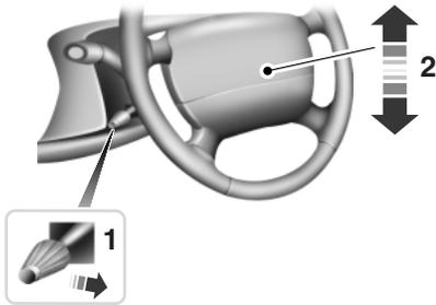
1. Pull and hold the steering wheel release lever.
