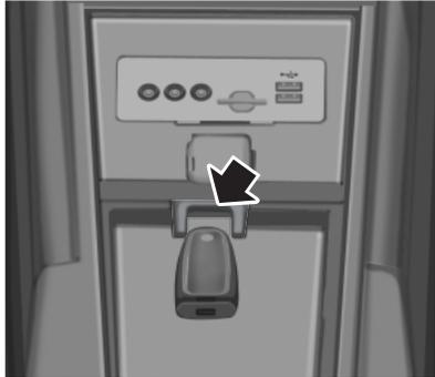
1. Locate the key backup slot at the front of the center console storage compartment.
