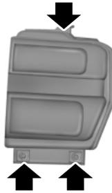
2. Remove the three screws from the headlamp assembly and pull the assembly straight out.
