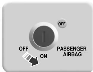
1. Insert the ignition key and turn the switch to on.
