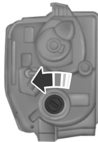
4. Remove the bulb assembly by turning it counterclockwise and pulling it straight out.
