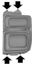
2. Remove the four screws from the headlamp assembly and carefully remove the lamp/bezel.
