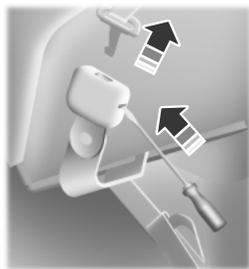
1. Disengage the lap and shoulder belt from the seat by inserting a key or small screwdriver into the slot in the detachable anchor and lifting upward (second row passenger side only).
