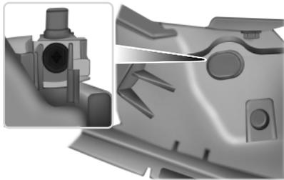
5. Locate the vertical adjuster on the back of each headlamp, then use a long Phillips #2 screwdriver to turn the adjuster either counterclockwise or clockwise in order to adjust the vertical aim of the headlamp. The upper edge of the light pattern should align with the horizontal reference line.
