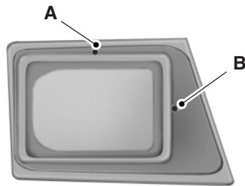
5. Locate the vertical adjuster (A) for each headlamp. Turn the adjuster control either clockwise or counterclockwise to adjust the vertical aim of the headlamp.
