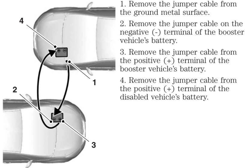
After the disabled vehicle has been started and the jumper cables removed, allow it to idle for several minutes so the engine computer can relearn its idle conditions.
