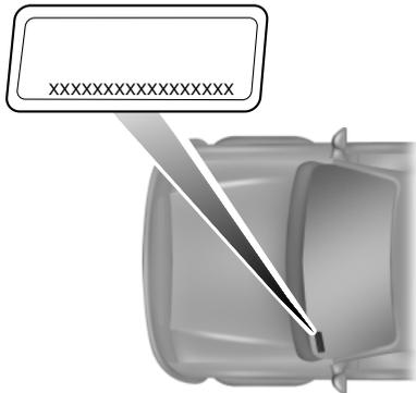
The vehicle identification number is located on the driver's side instrument panel.
