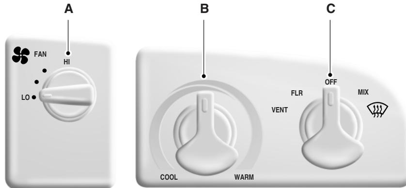
A. **Fan speed control:** Controls the volume of air circulated in your vehicle. Adjust to select the desired fan speed or switch off. If you switch the fan off, the windshield may fog up.
