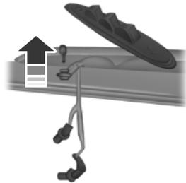
1. Remove the two screws from the high-mount brake lamp assembly and lift the lamp from the vehicle.
