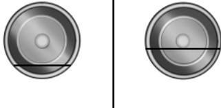
If driving through deep or standing water is unavoidable, proceed very slowly. Never drive through water that is higher than the bottom of the hubs (for trucks) or the bottom of the wheel rims (for cars).
