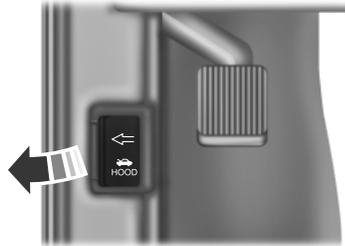
1. Inside the vehicle, pull the hood release handle located under the bottom left corner of the instrument panel.
