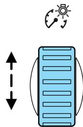
Move the control up or down to adjust the intensity of the panel lighting.
