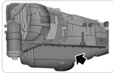
The TorqShift® automatic transmission is equipped with a serviceable transmission fluid filter located inside the transmission bottom pan.
