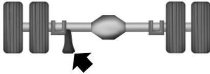
Rear axle jacking points - E-350 dual rear wheel and E-450
