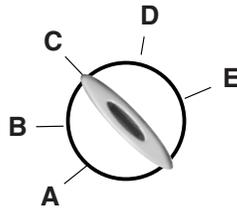
A. **Accessory:** Allows the electrical accessories, such as the radio, to operate while the engine is not running.
